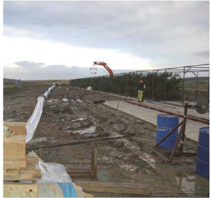
Figure 5: Large scale test set-up for effect of vegetation on explosion overpressure
