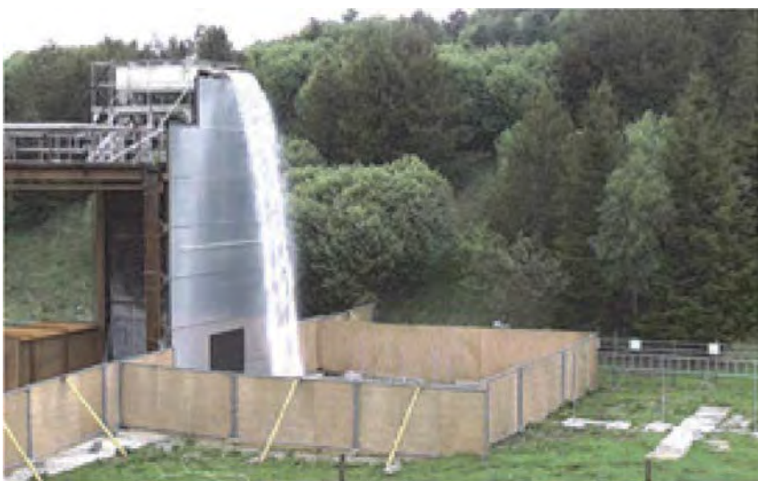
Figure 4: Liquid spills facility showing the test in progress (left) and the 1500 mm wide chute (right).
